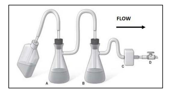
The left suction flask (A) is used to collect the contaminated fluids into a suitable decontamination solution; the right flask (B) serves as a fluid overflow collection vessel. An in-line HEPA filter (C) is used to protect the vacuum system (D) from microorganisms.
