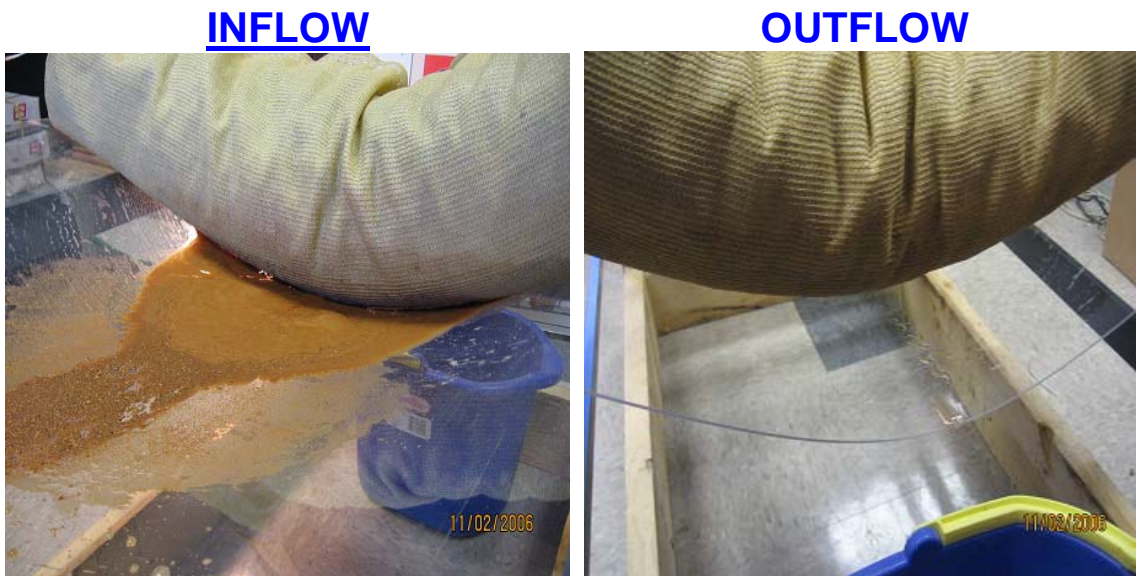
Figure 2 - Erosion EEL™ Surface Contact Test
