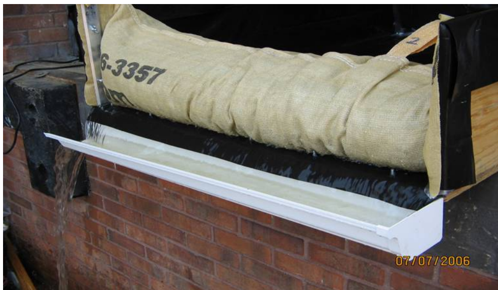
Figure 8 - Discharge from Flume Testing of Erosion Eel
